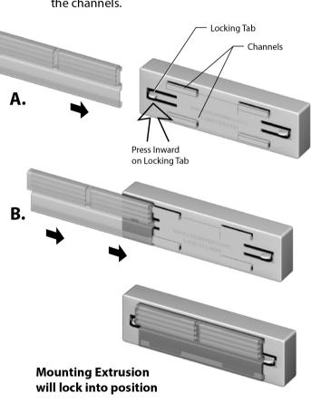
Attach Pricer and Extrusion onto the front of Pusher Shelf. **Note:** Align the notch on the Mounting Extrusion with the divider panel on pusher shelf.
