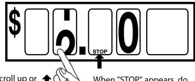
With finger tip, push scroll up or down until desired numeral appears, center in window. When "STOP" appears, do not scroll any further.
