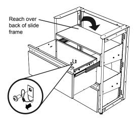
**5.** Open upper drawer. Reach over top of slide frame, grasp cable and thread through back of upper drawer, securing with screw.
