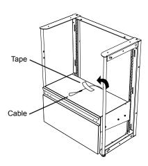
**3.** Close drawer, temporarily secure cable to top of drawer assembly with tape (not supplied).
