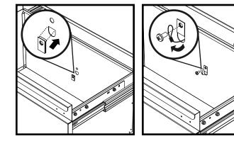
**2.** Open drawer, install screw clip. Thread cable through back of drawer and secure with screw.
