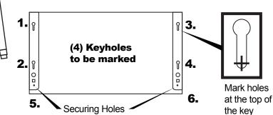
**C**- Carefully drill starter holes for the (6) wood screws
