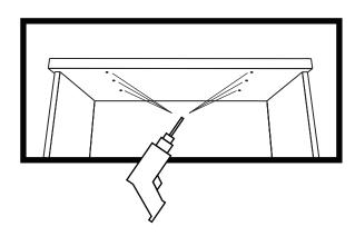
**D**Use screw driver to install the (4) screws into holes for keyhole slots. Do not tighten screws completely. Leave aproximately 1/8" gap between screw and surface.
