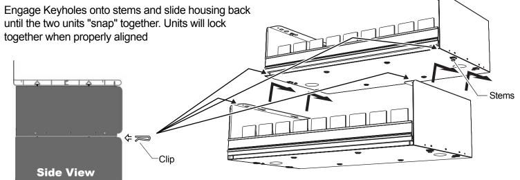
Push on the (2) securing "U" clips to secure the (2) under counter units together.
