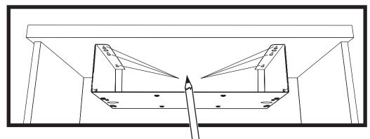
Temporarily position the pusher housing underneath the cabinet in the desired location.
